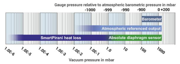
The VPM-7 functions as a genuine multi-sensor transducer featuring four pressure outputs that integrate a barometric ambient sensor, a wide-ranging heat-loss Pirani, an absolute diaphragm sensor, and a signal relative to atmospheric pressure. This combination is designed to enhance the pressure control capabilities of a contemporary load-lock vacuum chamber. Notably, the diaphragm sensor reading remains gas-independent within the absolute pressure range of 2 to 1333 mbar.
