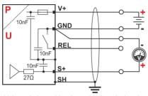
The high resolution 16-bit voltage signal can be interfaced to a PLC. A/D converter, voltmeter or other readout devices.
