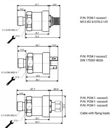
All dimensions are in mm unless otherwise stated - General tolerance ISO 2768-1 M 3D step files are available online at: www.sens4.com/support.html
