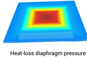
The piezo MEMS sensor consists of a diaphragm where one side of the diaphragm is exposed to the vacuum gas and the other side is exposed to a sealed reference vacuum. The applied pressure deflects the diaphragm and the deflection is converted to an electric signal.
