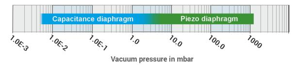
In vacuum applications where the gas composition or type can change, traditional gas dependent Pirani gauges will result in measurement deviation from the actual pressure. The VDM-5 transducer uses a precision ceramic capacitance diaphragm gauge (CDG) sensor and Piezo diaphragm sensor that eliminates the gas dependency and provides accurate measurements also when the gas properties change.
