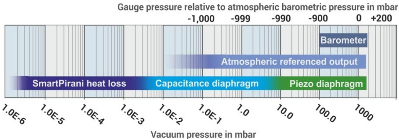
In environments where gas composition or type fluctuates, traditional gas-dependent Pirani gauges can result in measurement inaccuracies. The TriCAP™ ATM transducer integrates a high-precision capacitance diaphragm gauge (CDG) sensor, eliminating gas dependency and ensuring reliable measurements, even as gas properties change.
